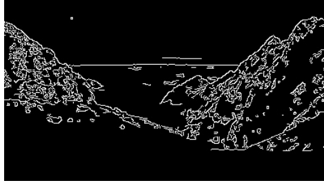
Figure 1.6: Sample output of canny edge detection method. As an input image we used figure 1.1
