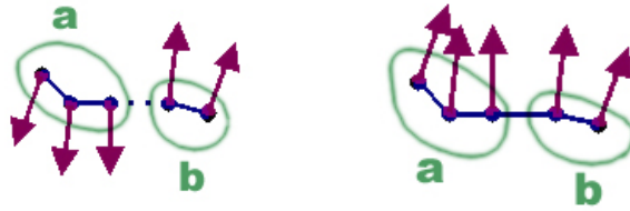
Figure 3.7: Normals Orientation Propagation
