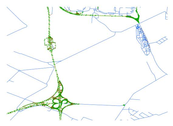
Figure 6.4: Amended graph using the short edges technique. Brown edges were added.
