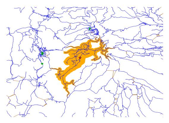
Figure 6.6: The isochrone (orange area) from starting point marked by a star, and a time limit of 6 minutes.
