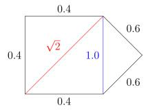
Figure 2.8: An example of the algorithm based on Hertel-Mehlhorn algorithm for minimal convex decomposition. The black pentagon represents the original graph face. The numbers denote the costs of traversing each edge. Triangulation added the red and blue edges.
