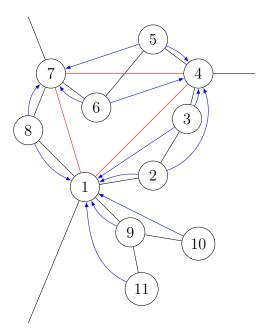
Figure 4.2: Example of creating the higher level graph from important roads. The black edges are the important road edges. Blue are the shortcuts from removed nodes. Red are the shortcuts that get added to the 2-core.
