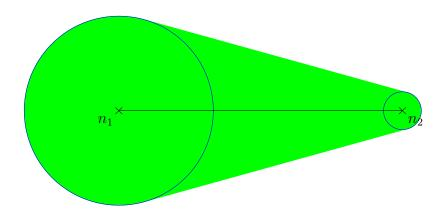
Figure 5.5: Convex hull used to approximate the union of circles when the whole edge is covered. The output is the convex hull of the two circles centered at  $n_1$  and  $n_2$ .
