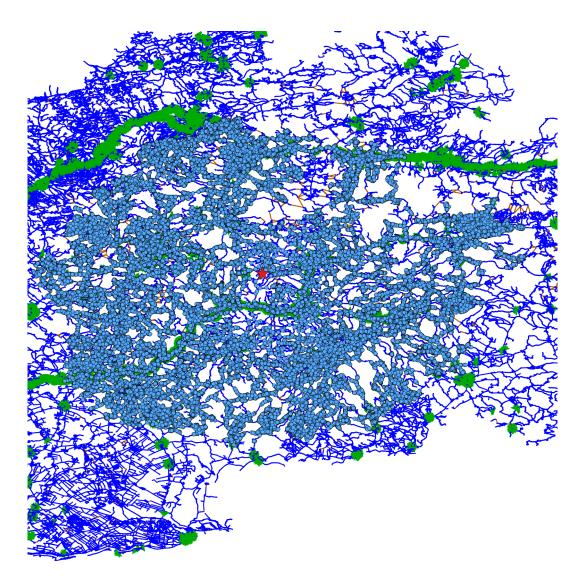
Figure 6.12: The nodes within isochrone found by the highway hierarchies algorithm.
