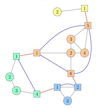
Figure 4.1: Example of creating the higher level graph. Original graph's edges are black. Cells are differentiated by background color of nodes. Red edges are the edges between cells. Border nodes are the squares. Blue edges are the shortcuts created by creating a clique between border edges of each cell. The higher level graph is made out of colored edges.
