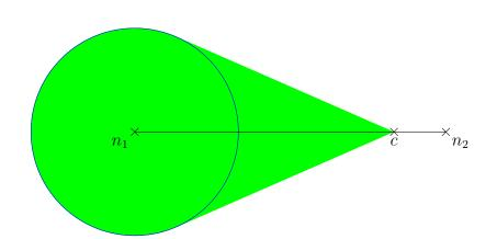
Figure 5.6: Convex hull used to approximate the union of circles when only a part of the edge is covered. The output is the convex hull of the circle centered at  $n_1$  and the point c.
