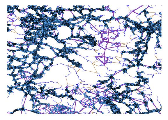
Figure 6.13: The nodes missed by the highway hierarchies algorithm. The higher level graph edges are purple. We can see that there are no edges going to the part of the road graph where the missing nodes are. This is because it is connected to the rest of the road graph using the added edges, which have relatively high cost.
