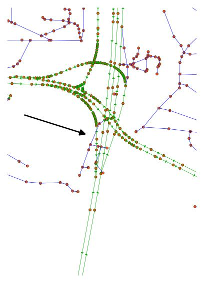
Figure 2.6: Example of intersections without node. There are intersecting edges where one is a bridge and the other is a road beneath the bridge. At 48.145N, 17.075E.
