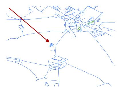
Figure 2.3: Example of disconnected map at 48.068°N, 17.249°E, the arrow points to a race track which is not connected to the road network.
