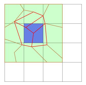
Figure 5.1: Our partitioning approach. The map is partitioned into squares. Then one square is selected (blue), with a buffer around it (green). This part of the map is partitioned. Cells that intersect the blue square (the red ones) are kept. Others (brown ones) are removed.
