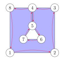
Figure 5.4: Face finding algorithm. Face is traversed counter-clockwise (red arrows).
