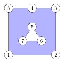
Figure 2.7: Example of a face in a road graph. Blue area is the road graph face.
