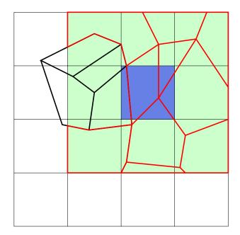
Figure 5.2: Second step of our partitioning approach (first step in figure 5.1). Next square with buffer is selected. This is then partitioned, while ignoring the parts of the map which were partitioned before (red is the new partition, black the partition from previous step).
