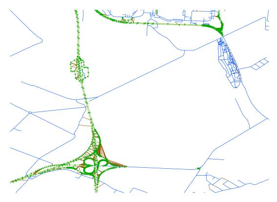
Figure 6.3: Amended graph using the triangulation technique. Brown edges were added.
