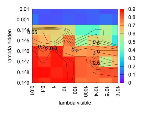
Figure 22: TLR performance on the *digits* task for  $\sigma = 1/\sqrt{784 + 1} \approx 0.036$  and  $\mu = 0.01$ . Best  $patSucc^F = 88.47\%$  with  $\lambda_v = 0.1$  and  $\lambda_h = 10^{-8}$ .
