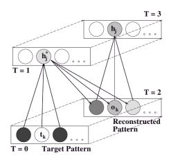
Figure 4: The recirculation algorithm by Hinton and McClelland (1988). Taken from (O'Reilly, 1996).
