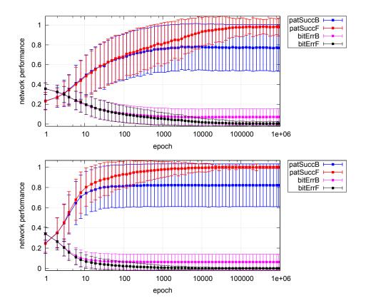
Figure 9: TLR success rate timeline for the 4-2-4 encoder task with  $\lambda_h = 0.0002$  and  $\lambda_v = 500$ . The top plot without candidate selection and the bottom plot with candidates selection.
