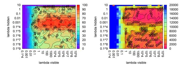
Figure 8: TLR success rate and convergence time needed for successful networks on the 4-2-4 encoder task with  $\sigma = 2.3$  and  $\mu = 0.0$ . Best network achieved 96.5\$ with  $\lambda_h = 0.0003$  and  $\lambda_v = 1000.0$ .
