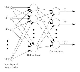
Figure 2: Fully connected feedforward *multi-layer* network with one *hidden* layer.
