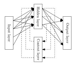
Figure 3: Simple recurrent network proposed by Elman (1990). Taken from Haykin (1994).
