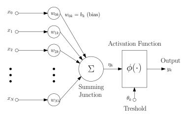
**Figure 1:** Perceptron transforming *inputs*  $[x_0, x_1, \ldots, x_N]$  to *output*  $y_k$ .
