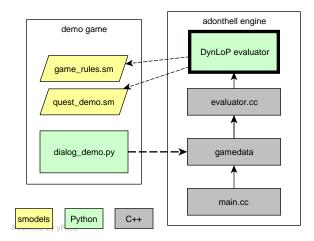
Figure 5.2: Integration of our DynLoP-WSE unit into Adonthell game engine. (C++ wrapper version)
