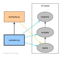
Figure 5.1: World state evaluator's component dependence scheme.
