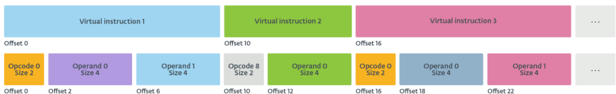
Figure 1. Illustration of bytecode, where all opcodes and operands are virtual
