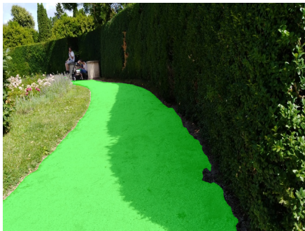
Figure: Prediction of driveable path - image resolution 640x480 on NVIDIA Jetson TX2.
