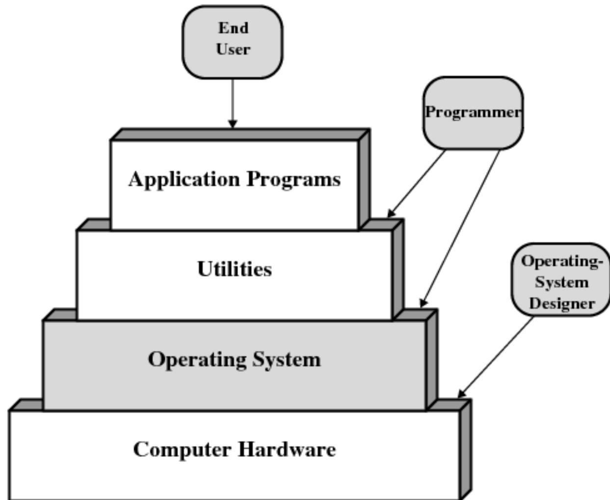
Figure 2.1 Layers and Views of a Computer System
