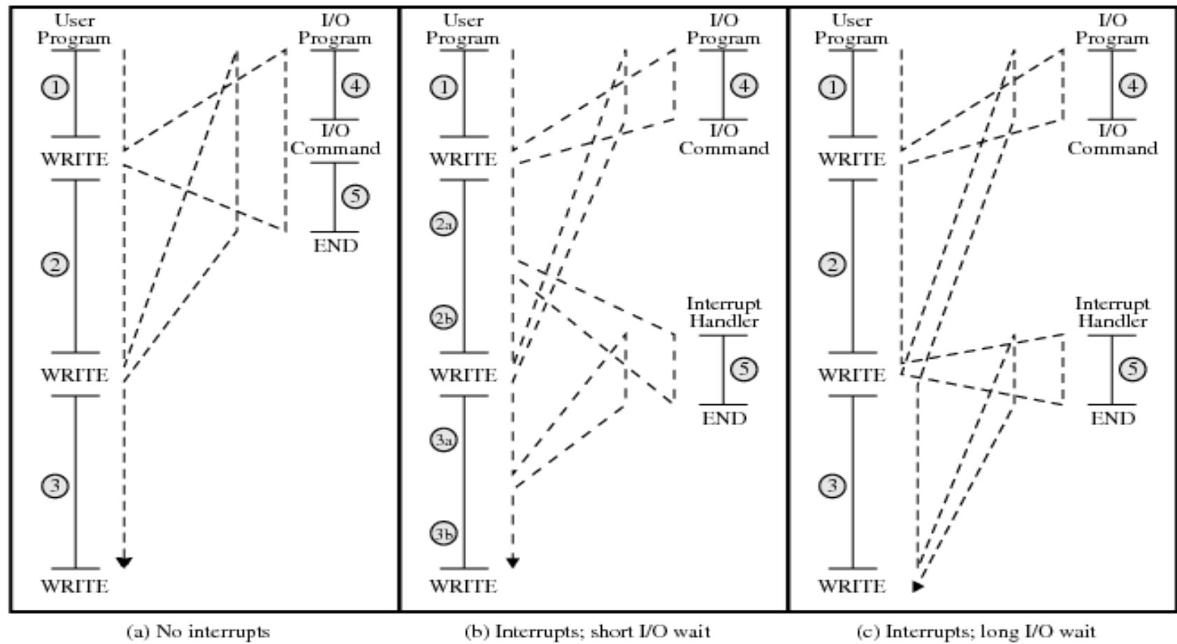
**Figure 1.5 Program Flow of Control Without and With Interrupts**
