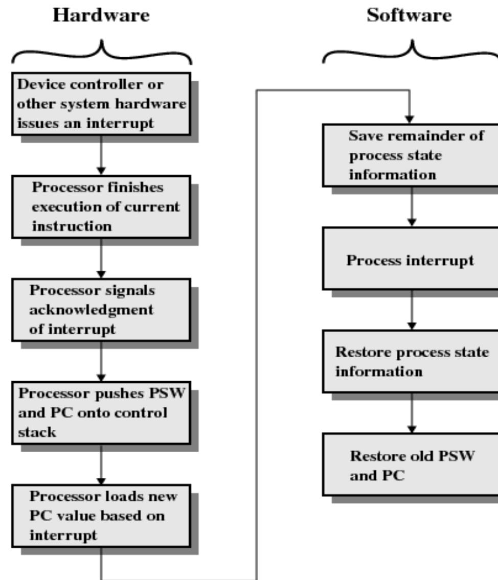
Figure 1.10 Simple Interrupt Processing
