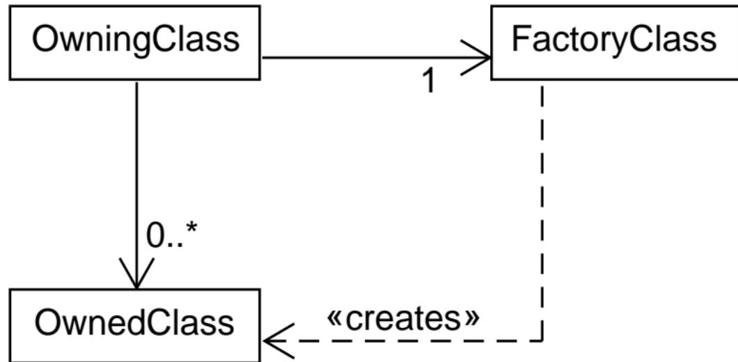
Composition gives rise to various problems in SW systems. Factory pattern is a standard way to eliminate it.
