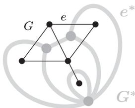
Fig. 4.6.1. A plane graph and its dual
